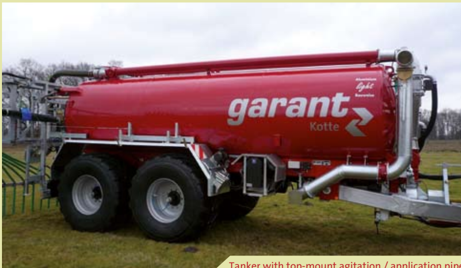
Tanker with top-mount agitation / application pipe
